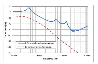
*Figure 1: Typical Common Mode and Differential Mode Attenuation provied by the filter as a function of frequency. Source and load resistance are*  $50\Omega$ .
